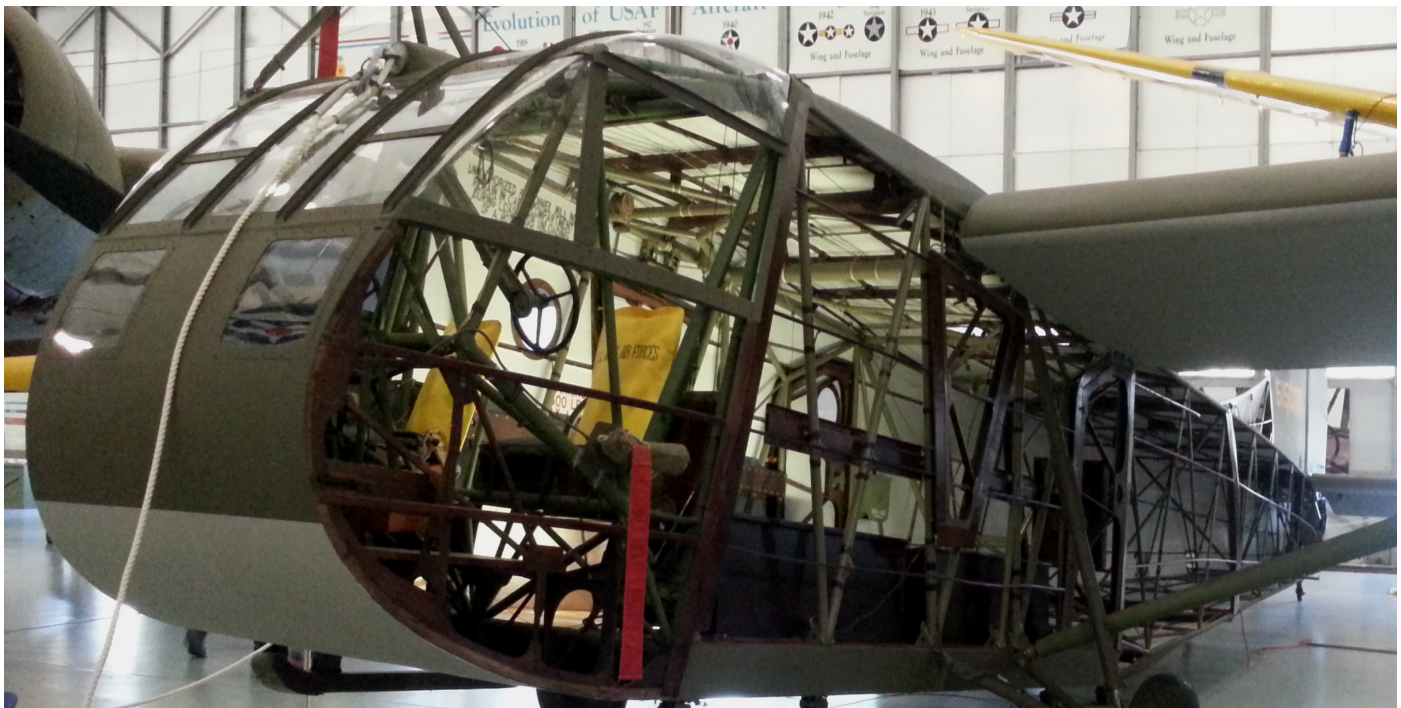
WWII combat glider: it's really made of wood and it's really, really big.
